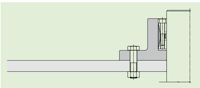
Brake disc connected with MAV 1008 and flange
