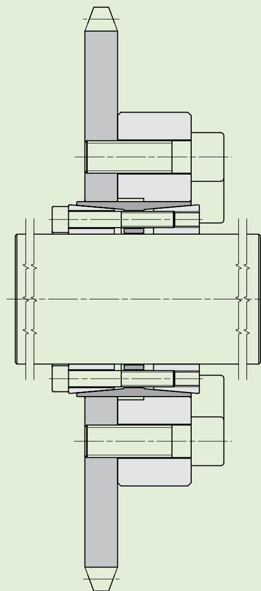
Pinion gear connected with MAV 4061. The resisting ring is used to compensate the pressure generated by the locking assembly in the zone adjacent to the pinion gear.
