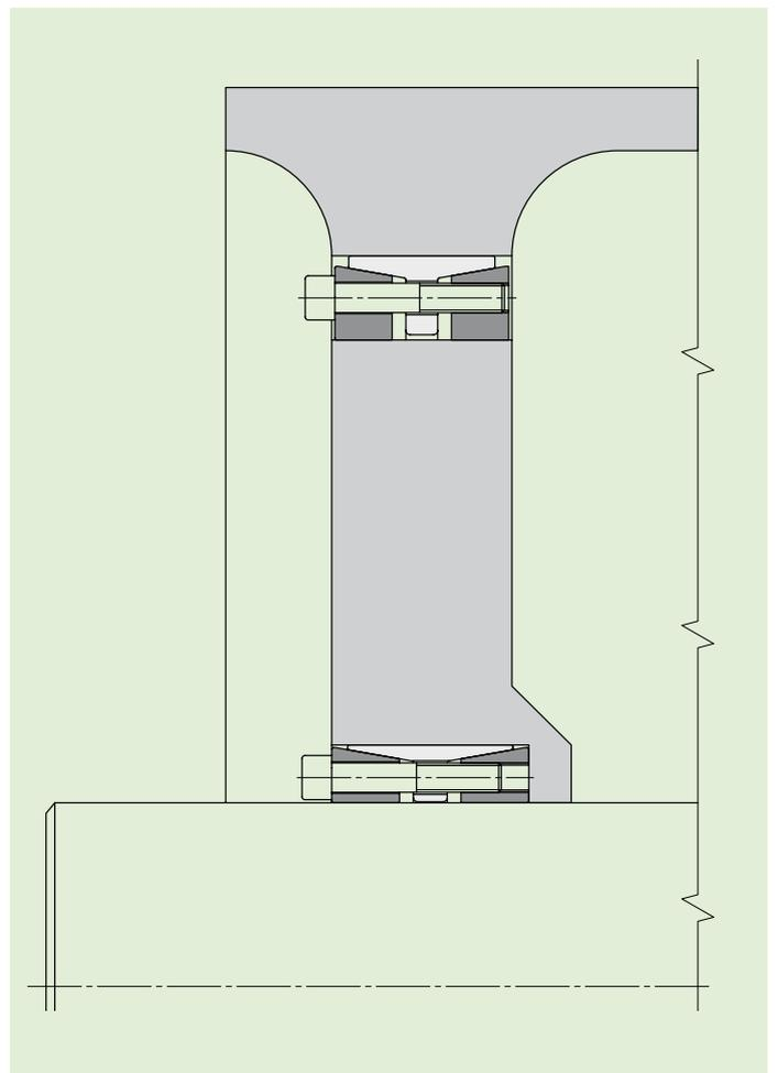
*Clay mill hub connected with two MAV 1008*
