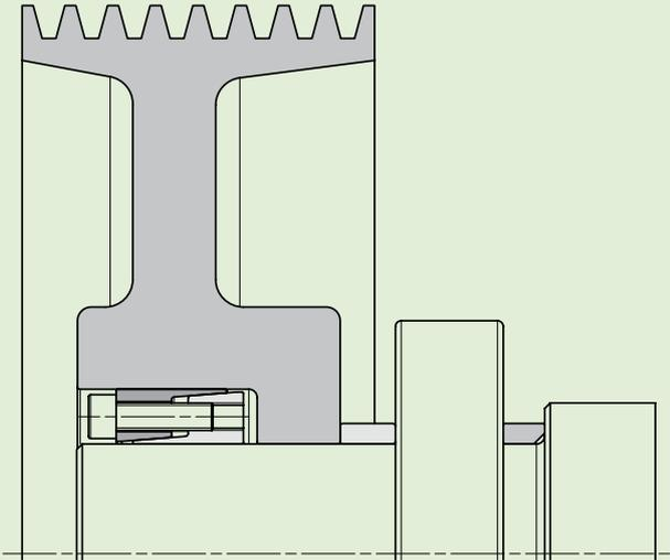
The specific purpose of series MAV 6903 is the axial locking of other elements adjacent to hub (e.g. bearings) during tightening of locking assembly. The movement of outer ring of locking assembly generates an axial force which is transmitted to hub and, by means of flanges and spacers, to adjacent elements.
