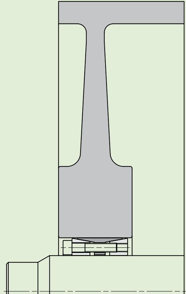
Connection of end disc of conveyor pulley for mining industry. The MAV 1008 allows an optimized “T” shaped design of the end disc, which is lighter and cheaper and compensates higher bending moment generated by the tension of the belt.
