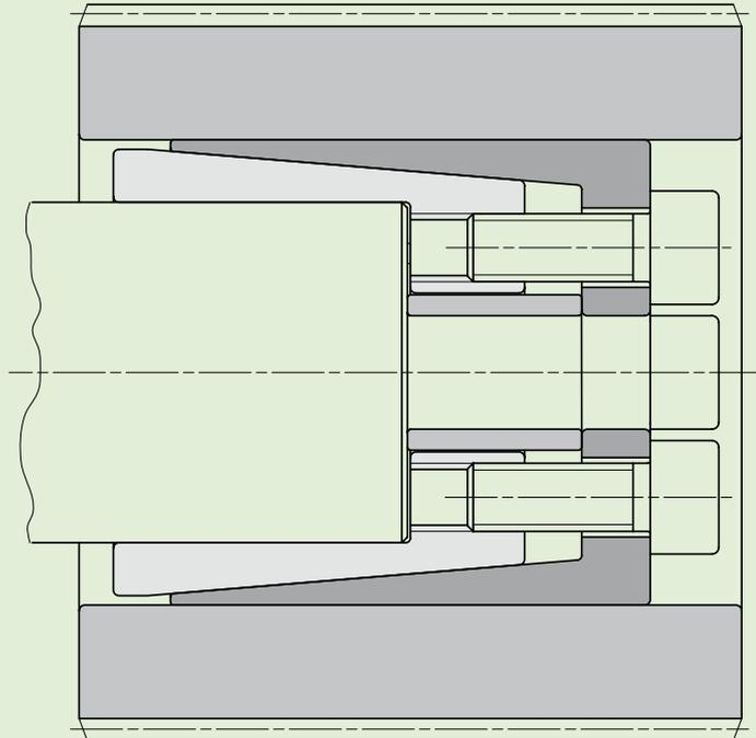
Special inverted MAV 5061 for connection of aluminum gear.
