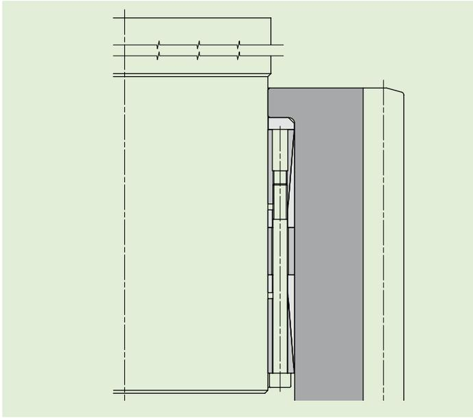
*Steel mill gear connected with special MAV 7061*
